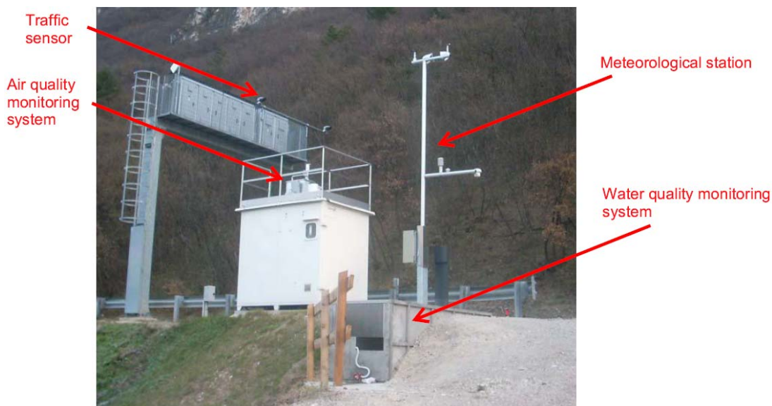
Figure 6: The first complete fixed monitoring site.
