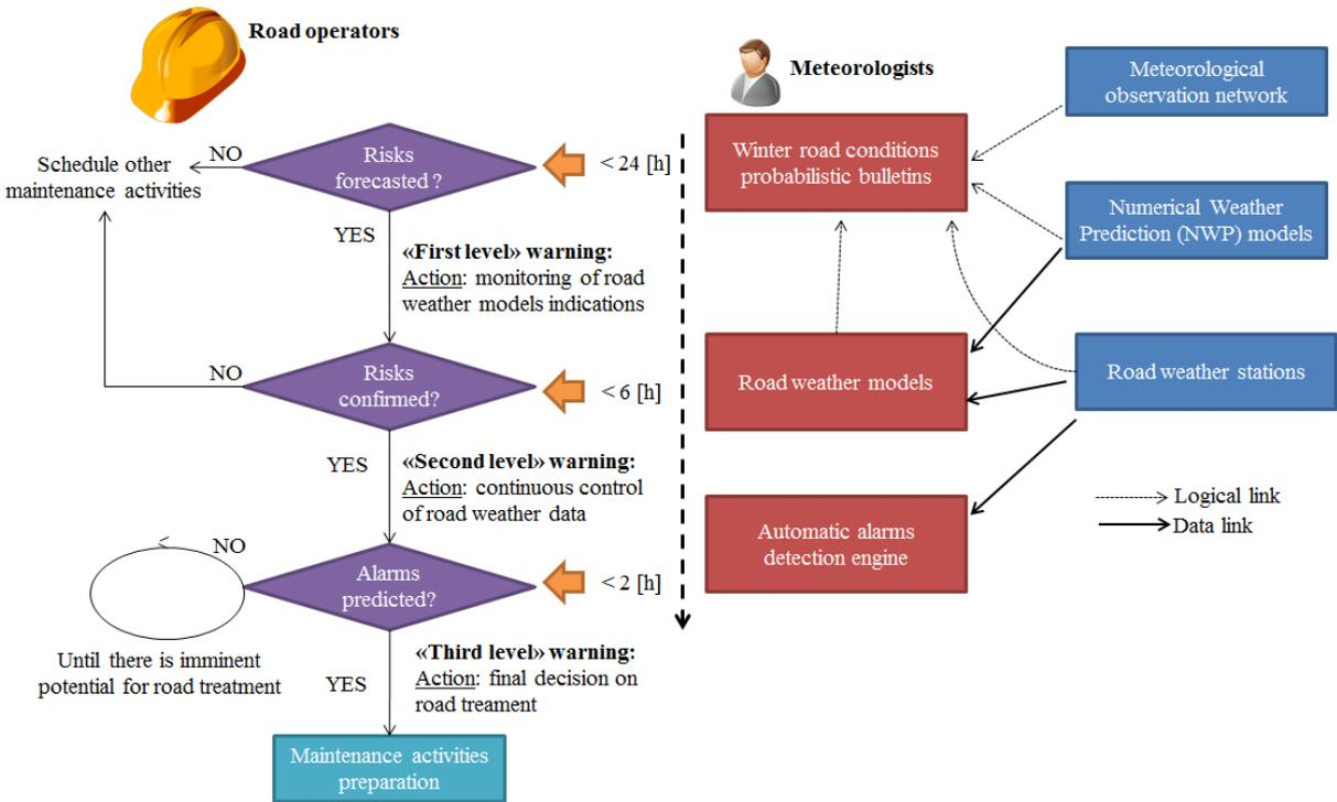
**Figure 4: The reference approach for the introduction of automated winter road management procedures.**
