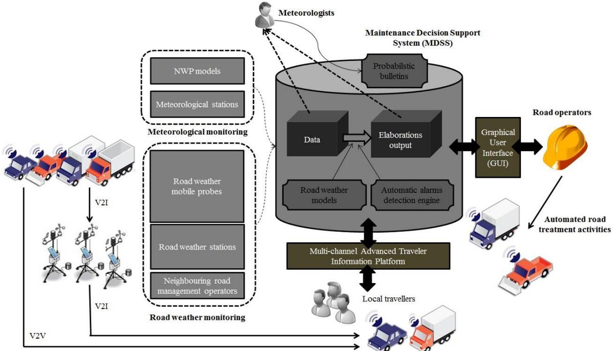
**Figure 6: Current (in grey) and future (coloured) CLEAN-ROADS architecture.**
