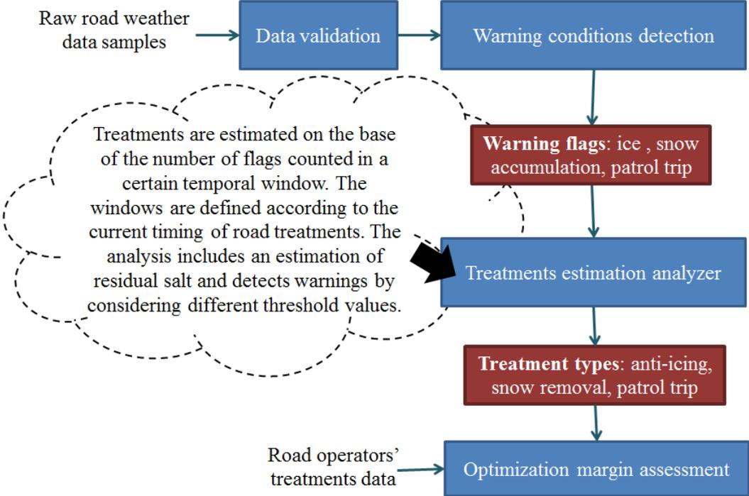
**Figure 2: The workflow for the estimation of optimal road treatments.**
