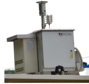
Figure 15: Air quality monitoring station.
