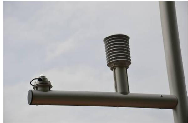
Figure 2: Pyranometer, thermometer and RH detector.
