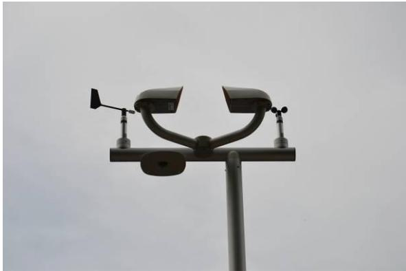
Figure 3: Anemometer, wind vane and precipitation detector.
