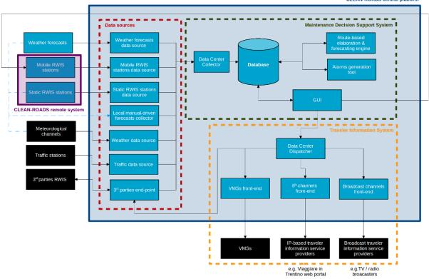
Figure 4: The high-level architecture of the CLEAN-ROADS system.
