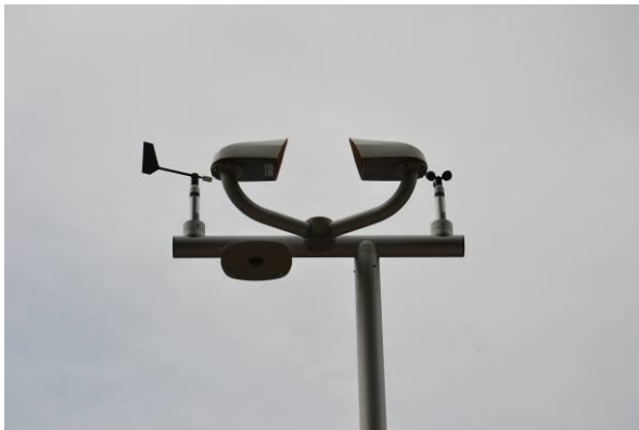
Figure 3: Anemometer, wind vane and precipitation detector.
