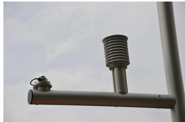
Figure 2: Pyranometer (left), thermometer and RH detector (right).
