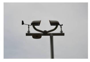
Figure 3: Anemometer, wind vane and precipitation detector.
