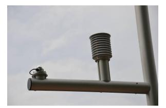
Figure 2: Pyranometer, thermometer and RH detector.
