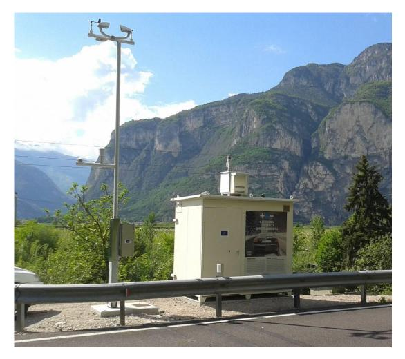
Figure 1: Typical configuration of RWIS station.
