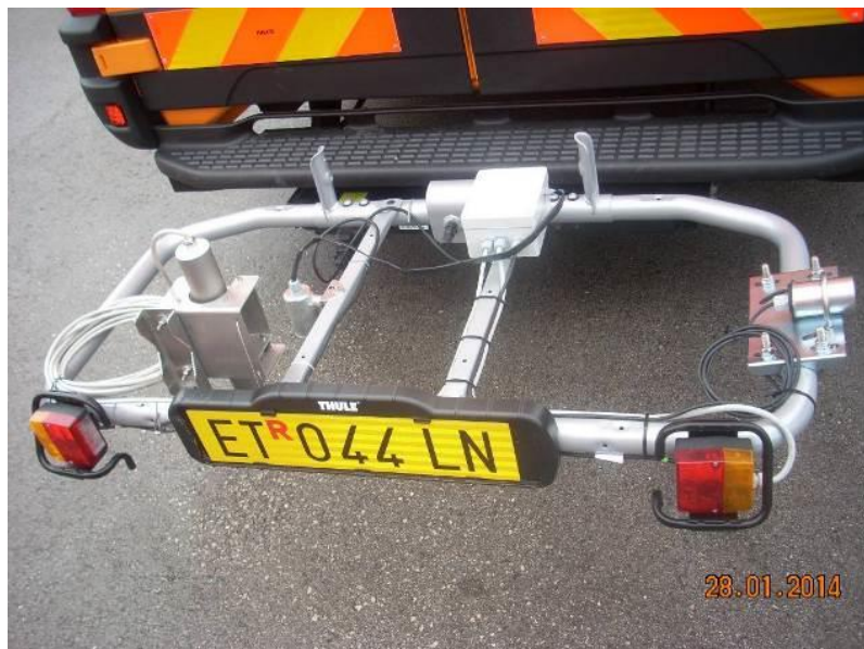
Figure 3: Mobile RWIS station prototype used during first field session activities in winter season 2013/2014.
